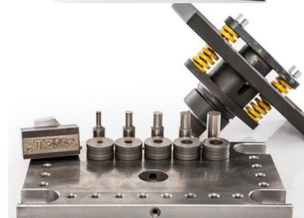
Accessory for performing technological undercuts for joining pipes at a 90-degree angle
